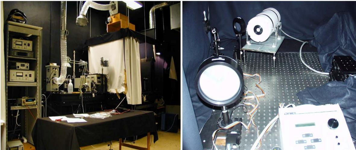
**Figure 2:** The spectral response characterization unit (Lamp and monochromator on the left, instrument, detector and mirrors in dark room on the right)
