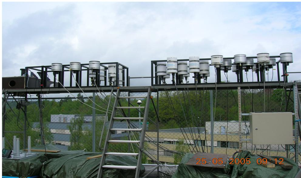
**Figure 1** : The solar platform with -mult-ifilter radiometers
